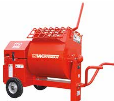
SWS-KLM45E & H WHITMAN 4.5 CUBIC FT MORTAR MIXER WM45E ELECTRIC OR WM45H GASOLINE POWERED WHEELBARROW STYLE MIXER DESIGNED FOR SMALL JOBS FITS 32" DOORS WT. 380 LBS
